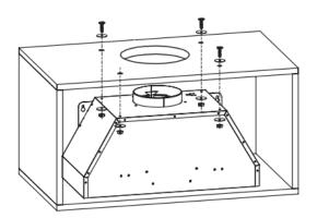
And then connect the ducting pipes to the outlet. Install the lamps and filter back to the hood.
